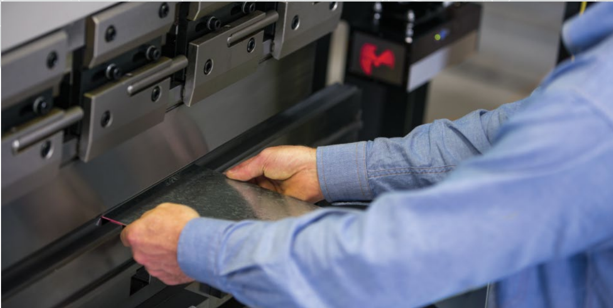
Close proximity protection enables safe handling of the work piece during high speed closing.
